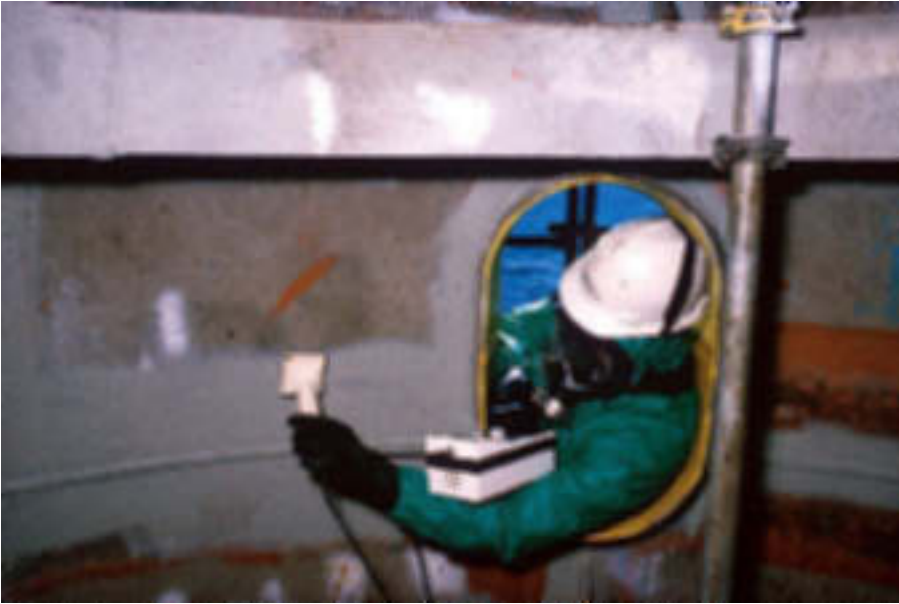
FIG. 30. NORM contamination within a vessel being measured using a surface contamination measuring instrument (courtesy: National Radiological Protection Board, UK).
