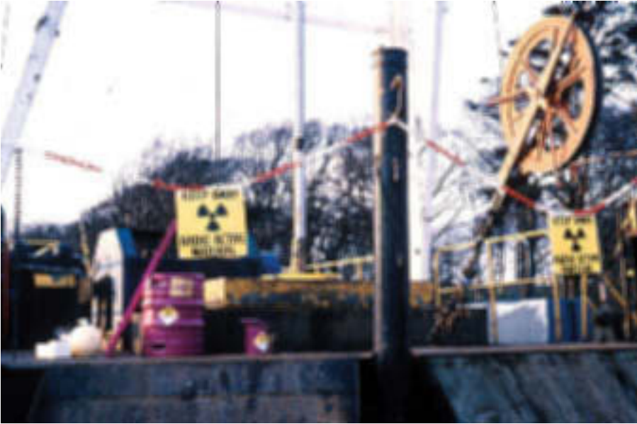
FIG. 17. Chain barriers designating a controlled area on the drill floor while logging sources are in use (courtesy: National Radiological Protection Board, UK).
